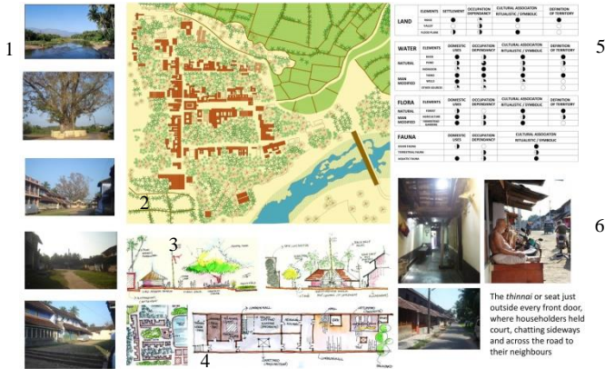
Figure 12: Documentation of A Tamil Brahmin settlement 1. Visuals,2. Plan grain,3. Sections,4. Typical residence plan, 5. Human nature interactions matrix, 6. Architectural spaces
