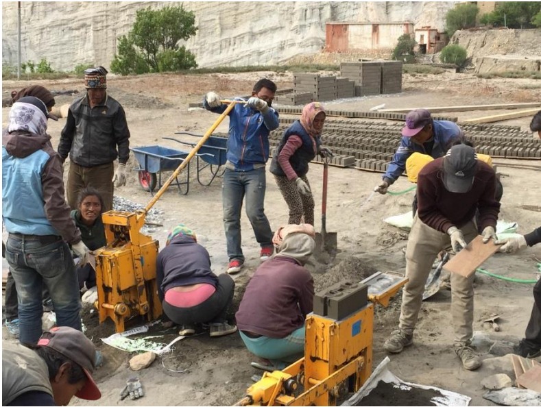
Fig. 6: Introducing compressed interlocked bricks at a workshop in Tetang
